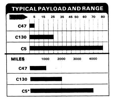
Aircraft designed for inter-theater airlift have a 13-fold increase in payload and a 6-fold increase in capacity over their WW II predecessors. With the C5, tanks, APCs, artillery pieces, and helicopters can be airlanded overseas in hours. All in all, considering payload, range, and speed, the C5 is 100 times more productive than its World War II counterpart, the C47.
