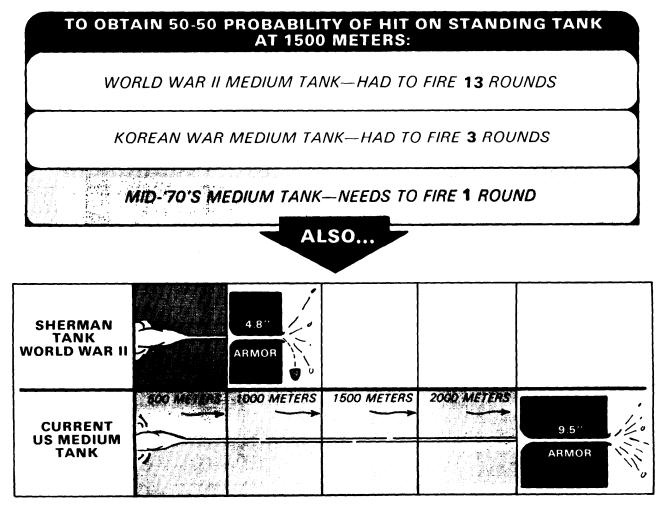
The Sherman tanks of General Patton's Third Army had to close to within 500 meters of the German PzV Panther tank before the American 76mm gun could punch through the German's 4.8 inches of frontal armor. Current US medium tanks can penetrate nearly *twice* that much armor at *four times the range*.
